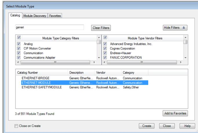
4. Press Create, then the new module window will appear and you can enter the Name of the Module, IP address, and the connection parameters as shown in the screen shot. Note: Configuration = 1, 0 (8-bit)
