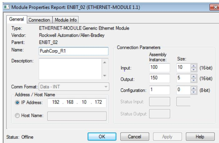
Note: Input and Output should be set to 16-bit
